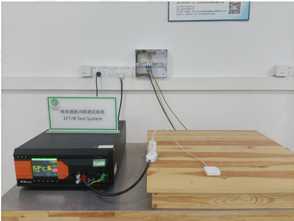
Photographs 8: Set-up for Electrical fast transient (EFT)
