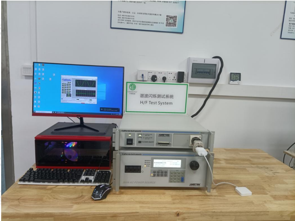
Photographs 5: Set-up for Voltage fluctuations & flicker
