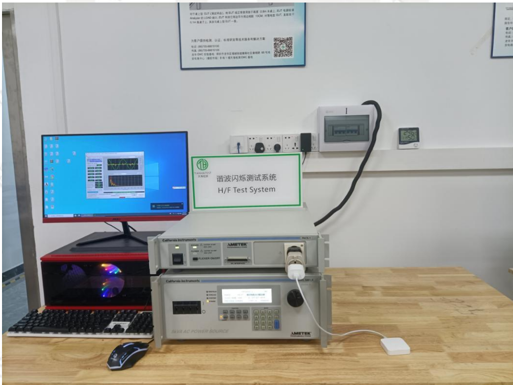
Photographs 4: Set-up for Harmonic current emissions
