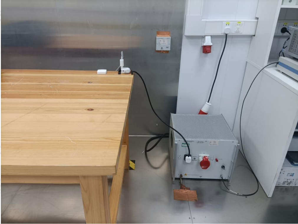
Photographs 1: Set-up for Conducted disturbance at mains terminals
