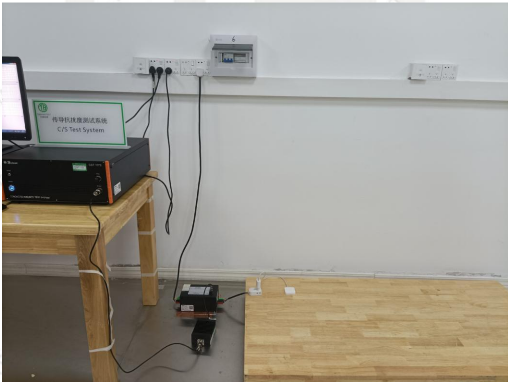
Photographs 10: Set-up for Radio-frequency, Continuous conducted disturbance (CS)
