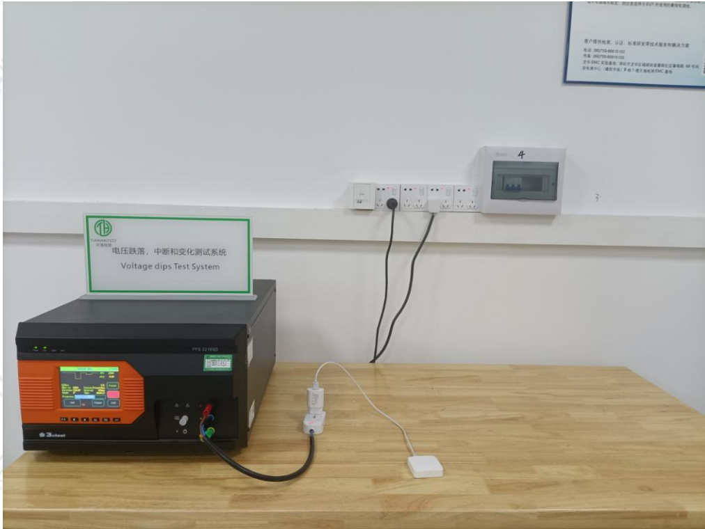
Photographs 11: Set-up for Voltage dips & Voltage interruptions
