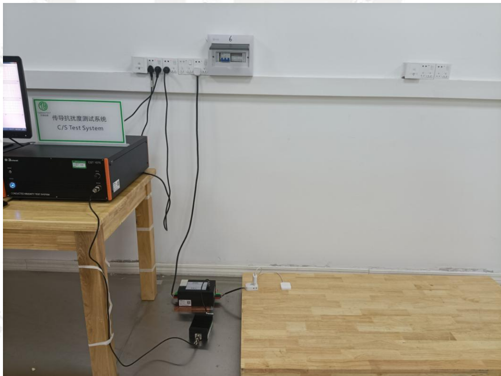
Photograph 8: Set-up for Conducted disturbances, induced by radio-frequency fields
