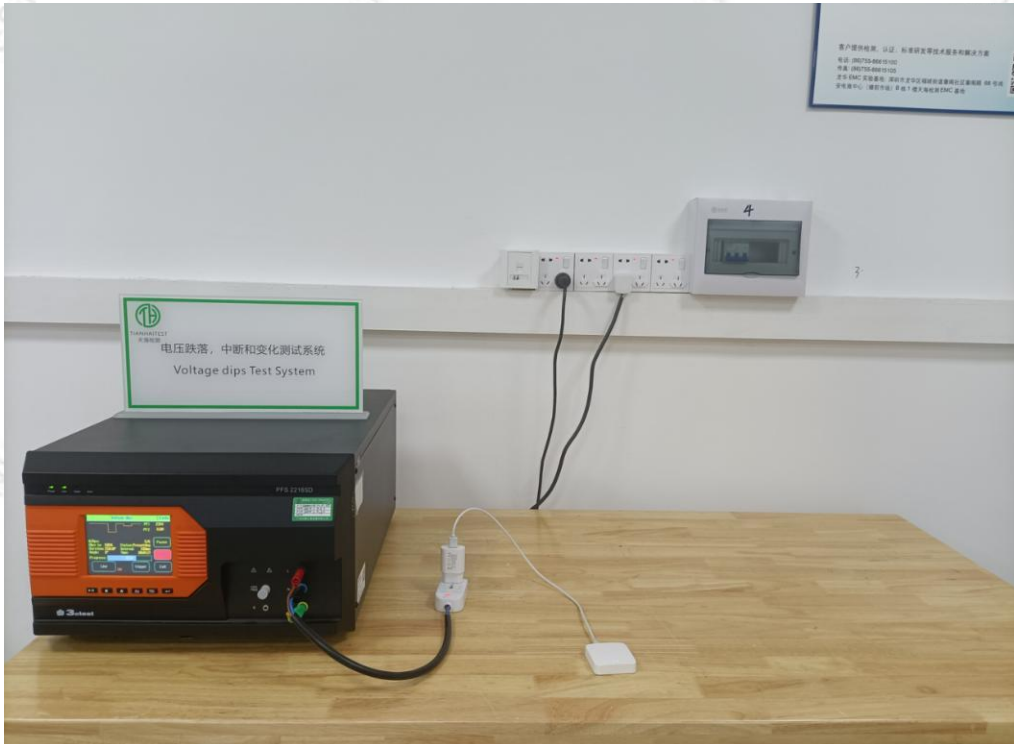
Photograph 9: Set-up for Voltage Dips and Interruption
