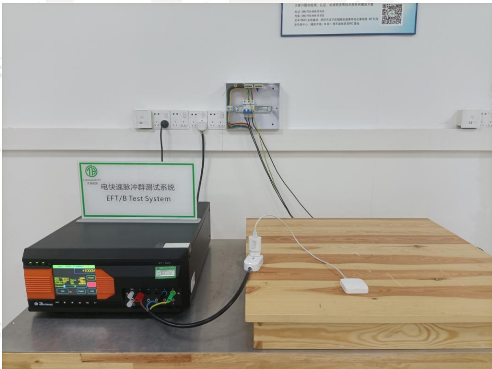
Photograph 6: Set-up for Electrical Fast Transient / Burst
