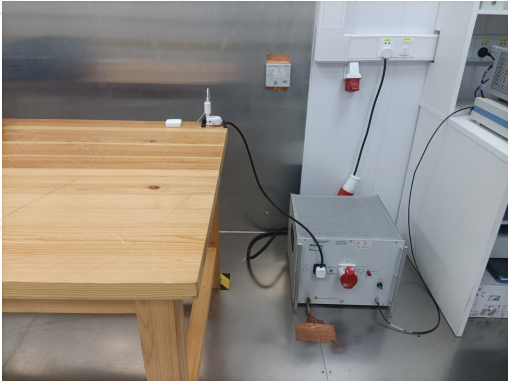
Photograph 2: Set-up for Radiation Emission (Below 1GHz)
