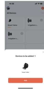
Option 1: Long press the manual button on water valve for 5s until the indication wifi blue light in quick flash, then you can see the device pop up in APP to be added, press ADD to finish connection.
