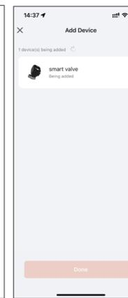
Option 2: When device is under connection status, click + in right upper corner to add device, choose "water valve" from Industry & Agriculture, then the app start to scan the devices around, you can choose correct device and add by steps.
