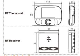
The installation distance between the thermostat and the receiver does not exceed 200m (the distance can be judged according to the actual network coverage)
