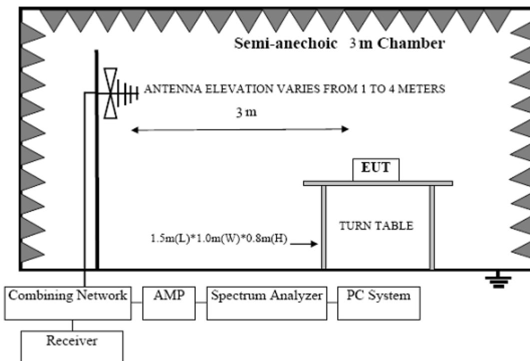
Semi Anechoic Chamber (3m) Test Setup Diagram for Above 1GHz
