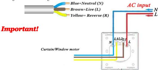
Note: The motor blue wire is Neutral line. Motor blue wire to Switch N port always. Brown for L1 and Yellow for L3, or connect Brown to L3 and Yellow to L1 to change open direction.
